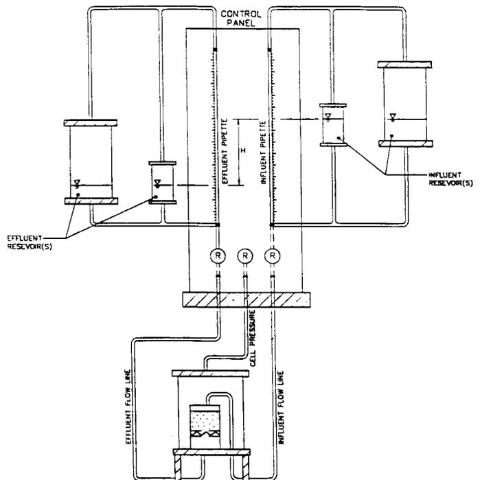
FIG. 1 Schematic Diagram of HCR Test Equipment
